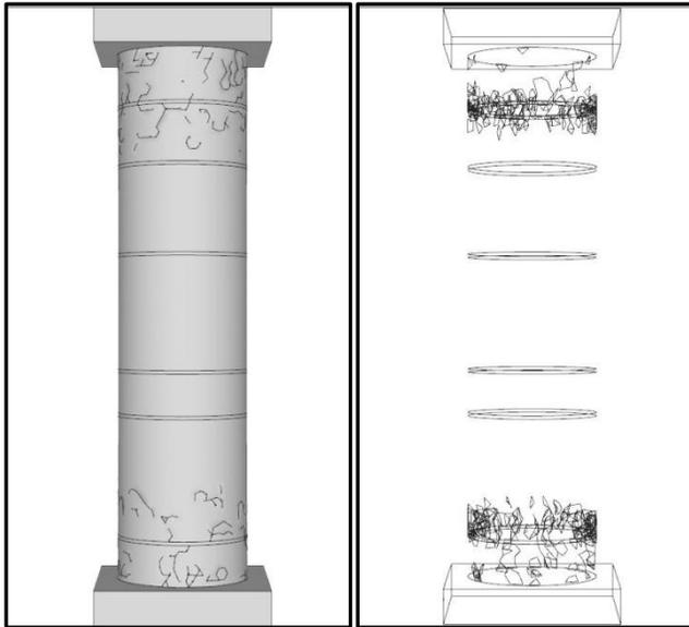
*b- Fracture propagation at its initial stages.*
