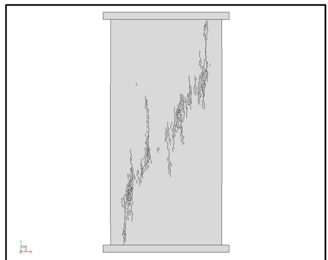
d- Fracture pattern at its final stages.
