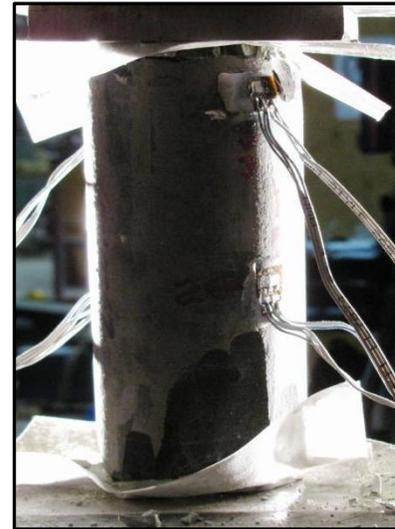
Fig. 8. Montney sample failed throughout the UCS test.
