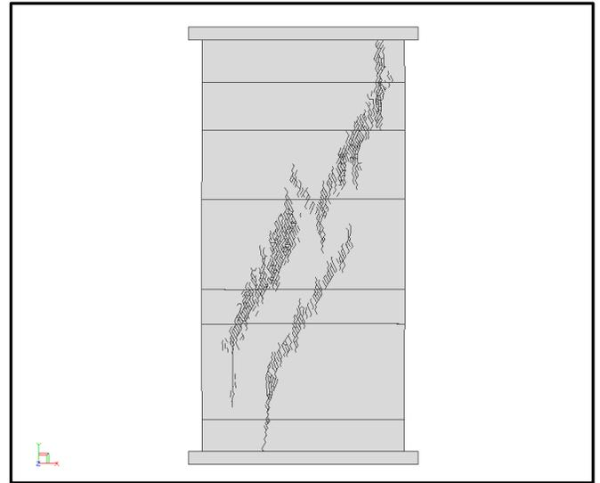
d- Fracture pattern at its final stages.
