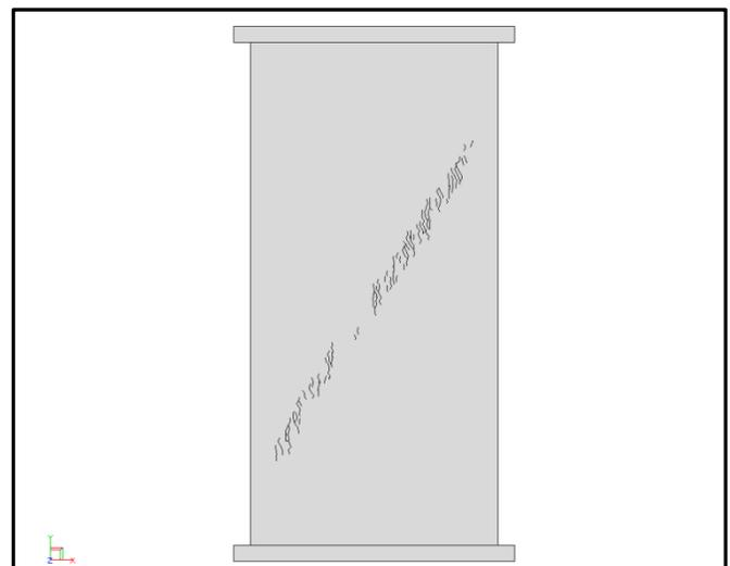
c- Fracture pattern at its initial stages.
