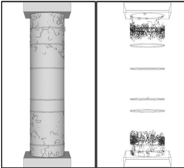
*c- Fracture propagation at its final stages.*
