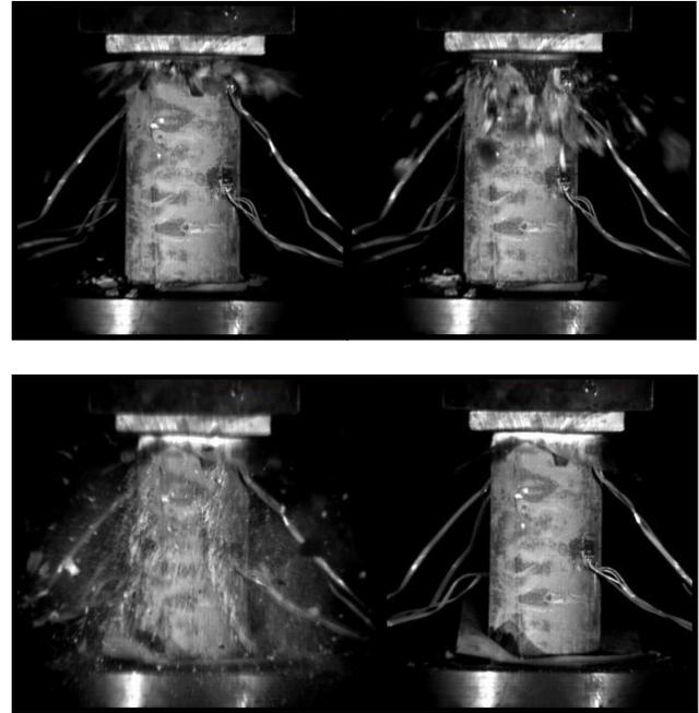
Fig. 7. Failure progress in Montney shale under UCS test [13].
